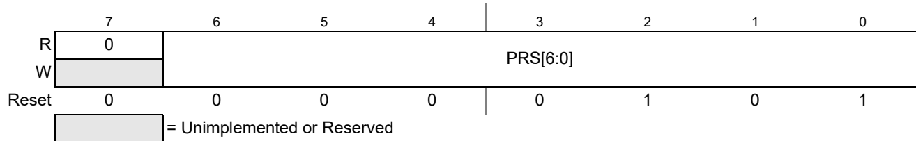
Figure 9-7. ADC Timing Register (ADCTIM)
