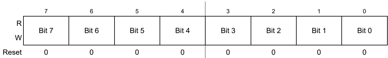
Figure 12-19. Timer Input Capture/Output Compare Register x Low (TCxL)
