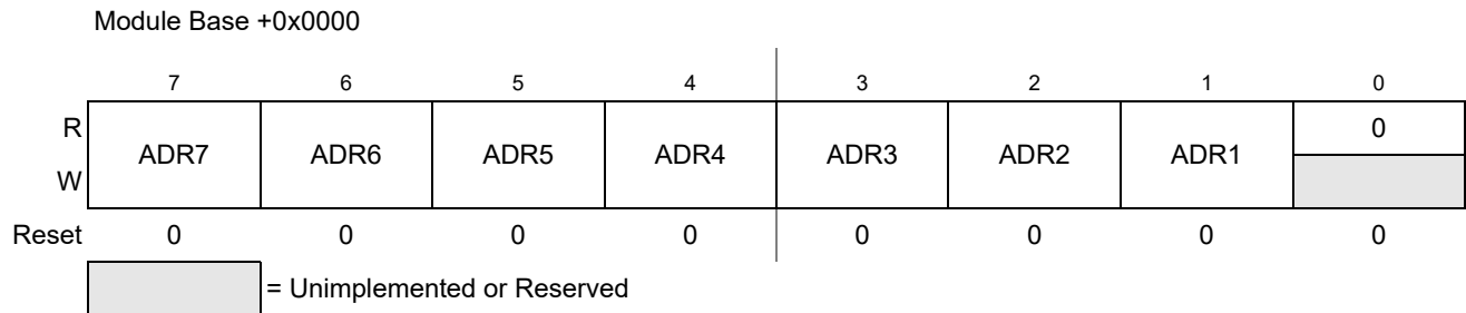
Figure 16-3. IIC Bus Address Register (IBAD)
