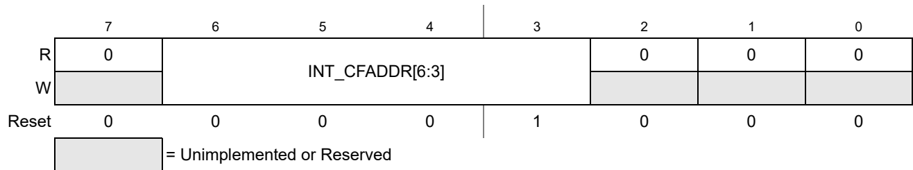
Figure 5-4. Interrupt Configuration Address Register (INT_CFADDR)
