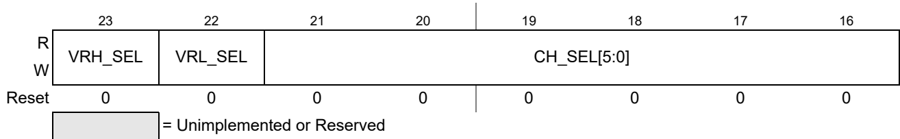
Figure 9-19. ADC Command Register 1 (ADCCMD_1)
