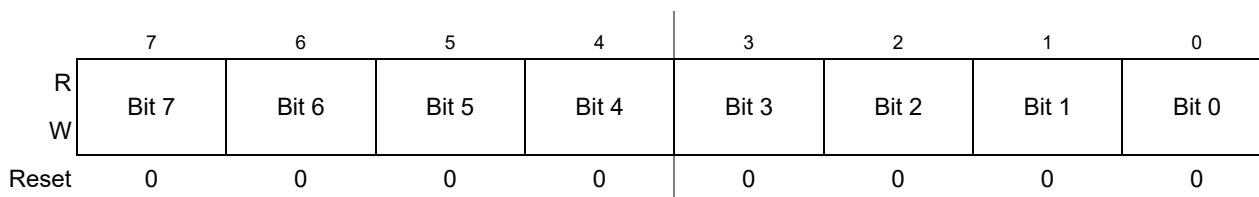
Figure 11-23. Timer Input Capture/Output Compare Register x Low (TCxL)
