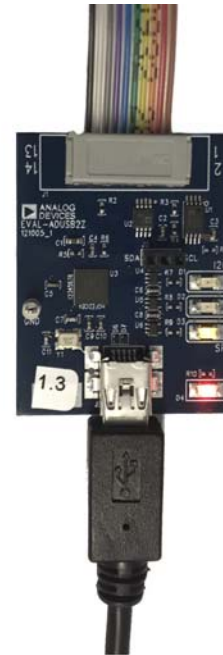
Figure 7. State of the USBi Status LEDs After Driver Installation
