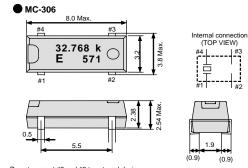
Do not connect #2 and #3 to external device. The metal case inside of the molding compound may be exposed on the top or bottom of this product. This purely cosmetic and does not have any effect on quality, reliability or electrical specs.
