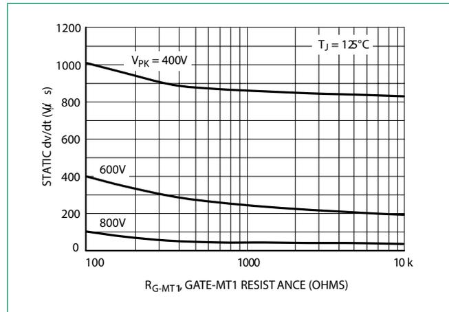
**Figure 9. Exponential Static dv/dt vs. Gate-MT1 Resistance, MT2(+)**
