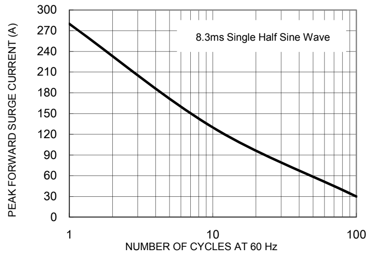
FIG. 5 MAXIMUM NON-REPETITIVE FORWARD SURGE CURRENT
