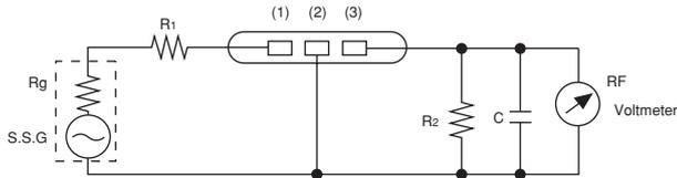
$R_g + R_1 = R_2 =$  Input and Output Impedance
