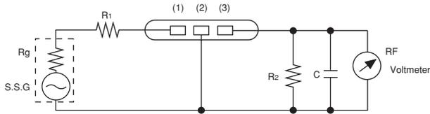
$R_g + R_1 = R_2 =$  Input and Output Impedance
