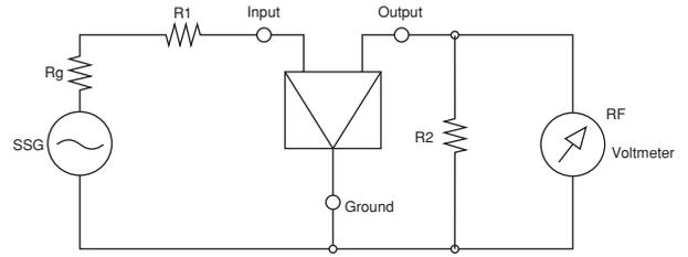
$R_g + R_1 = R_2$  : Input/Output Impedance
