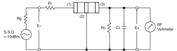
$R_g = 50\Omega$     $R_1 = 280\Omega \pm 5\%$     $R_2 = 330\Omega \pm 5\%$
