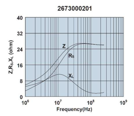
Impedance, reactance, and resistance vs. frequency.
