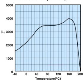
Measured on a 17/10/6mm toroid at 10kHz.
