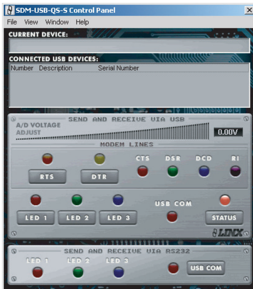
Figure 12: The Control Panel for RS-232 Operation
