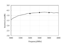
3400 MHz -0.80 dB 3600 MHz -0.70 dB 3800 MHz -0.71 dB
