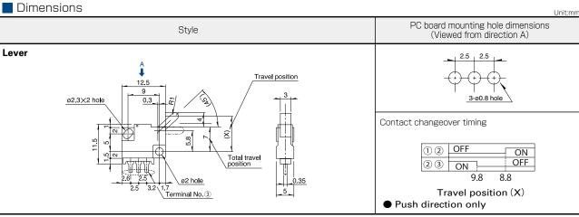
Dimensions drawing is for PC board terminal type.
