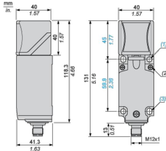
(1) 2 holes Ø 5,45 mm / Ø 0.21 in. (Tightening torque: < 1,5 Nm / < 13.3 lb-in.)
