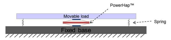
By applying a voltage to the actuator, it elongates and therefore moves the load. This movement can be felt by the user. For a maximal haptic feedback, the rear panel needs to be as heavy as possible. Otherwise the PowerHap actuator will not only move the load but also the rear panel and therefore a part of the performance is lost.
