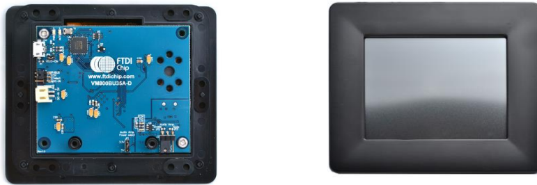
Figure 3-1 - VM800BU module profile 3.5" display version
