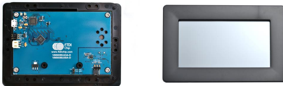
Figure 3-2 - VM800BU module profile 4.3" display version
