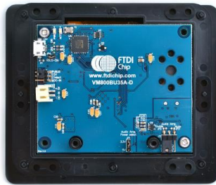
Figure 3-1 - VM800BU module profile 3.5" display version
