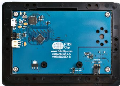
Figure 3-2 - VM800BU module profile 4.3" display version
