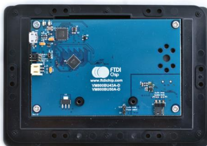
Figure 3-3 - VM800BU module profile 5" display version
