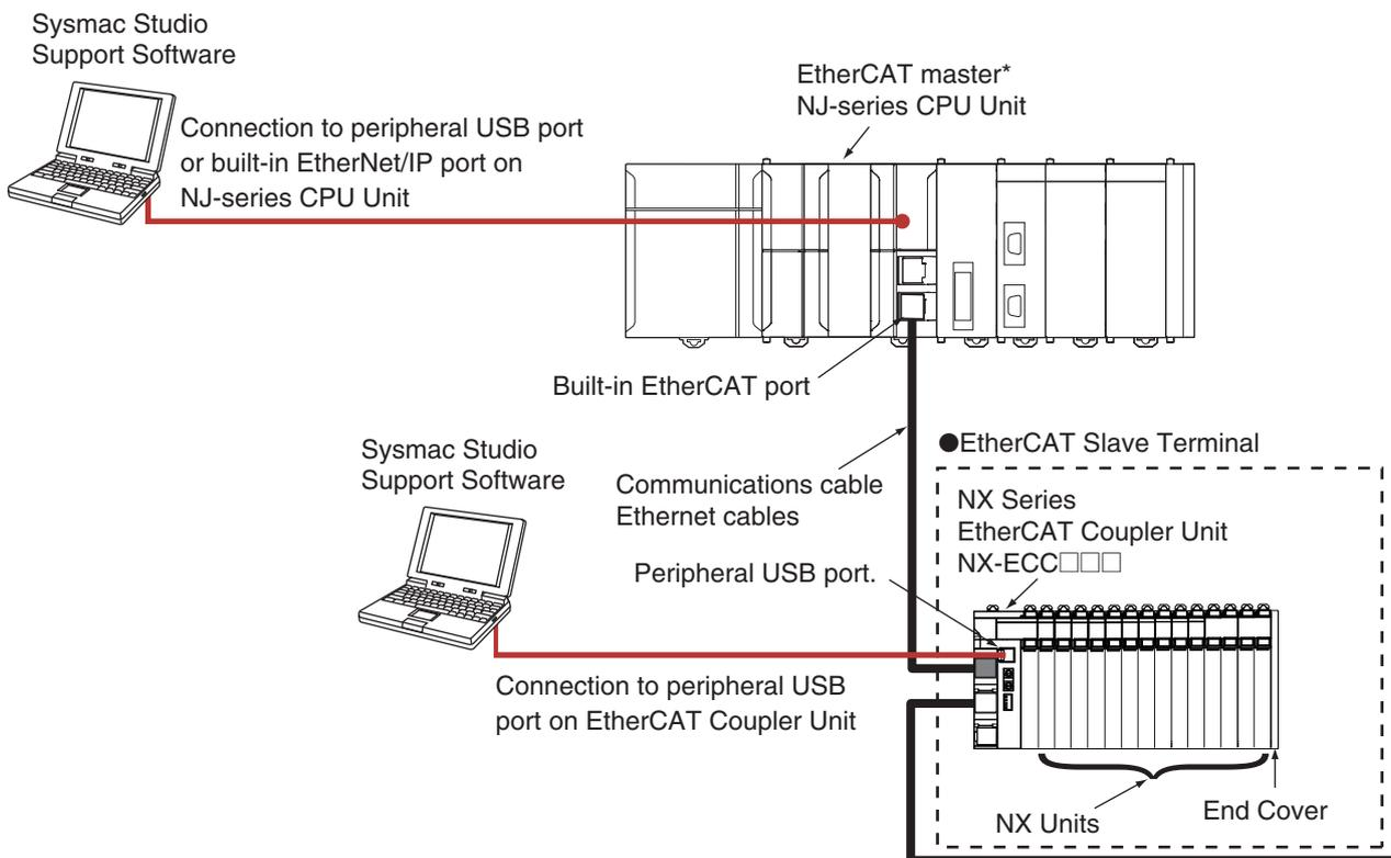
\* OMRON CJ1W-NC□81/□82 Position Control Units cannot be connected to the EtherCAT Slave Terminal even though they support EtherCAT.
