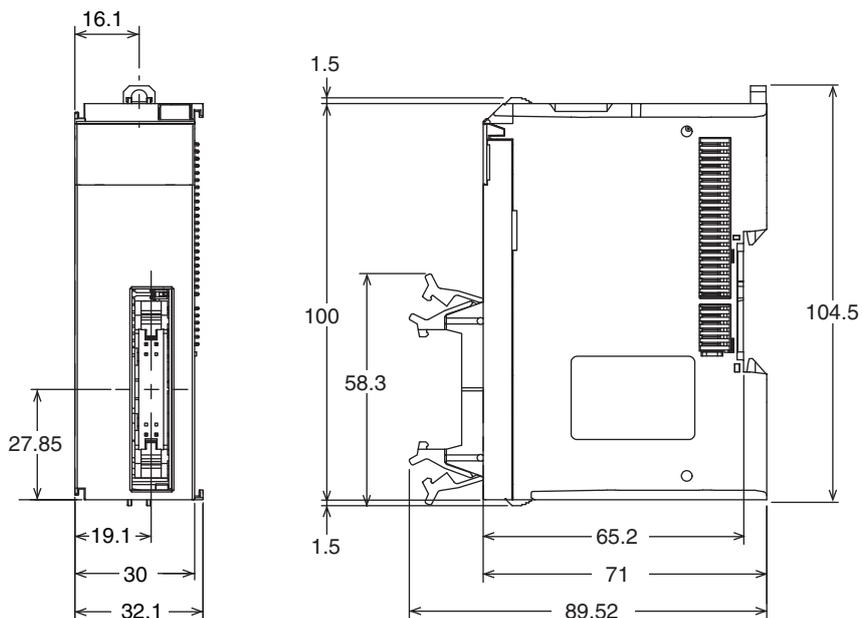
**Units with MIL Connectors (1 Connector with 40 terminals)**
