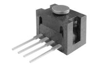
**Leadership, in full force.** Whether it's critical applications such as IV drips or dialysis, or serious engineering like robotic end-effectors, Honeywell Sensing and Internet of Things (SIoT) offers an unbeatable line of force sensor options. These sensors measure the addition or backup of force — meaning, the resistance of silicon-implanted piezoresistors increases when flexed under applied force. Each sensor concentrates force
