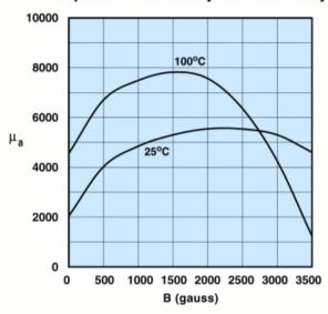
Measured on an 18/10/6mm toroid at 10kHz.
