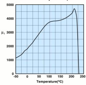
Measured on an 18/10/6mm toroid at 100kHz.
