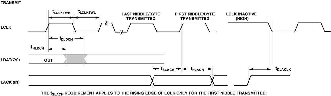
Figure 23. Link Ports—Transmit
