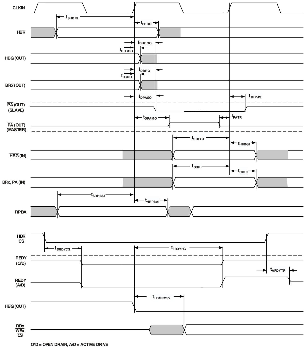
Figure 17. Multiprocessor Bus Request and Host Bus Request
