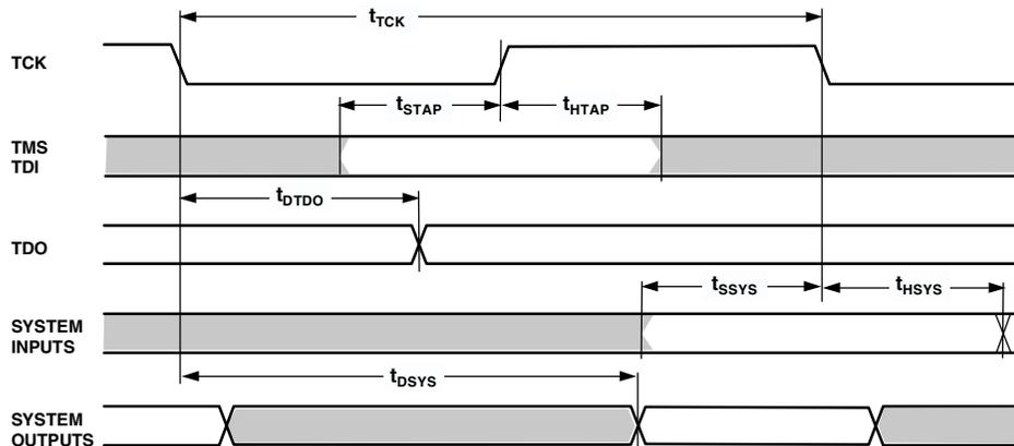
Figure 26. JTAG Test Access Port and Emulation
