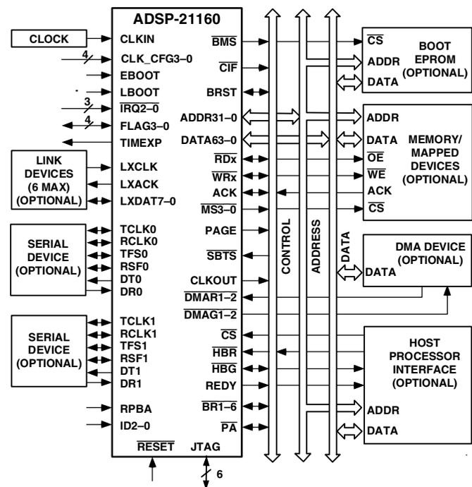
Figure 1. Single-Processor System
