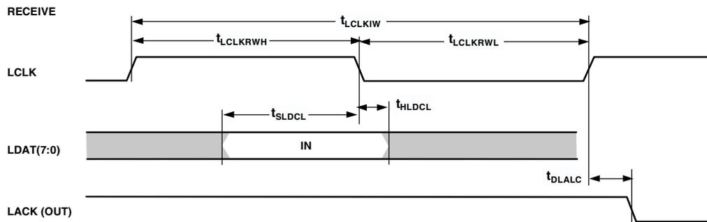
Figure 22. Link Ports—Receive
