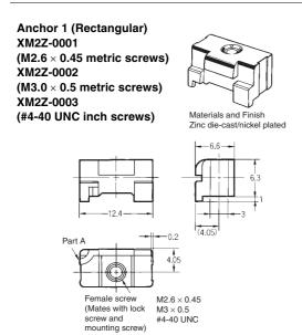
Note: When using a Dust Cover, secure the holding ring at part A.
