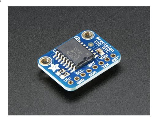
The datasheet for the DS3231 explains that this part is an "Extremely Accurate  $I^2$ C-Integrated RTC/TCXO/Crystal". And, hey, it does exactly what it says on the tin! This Real Time Clock (RTC) is the most precise you can get in a small, low power package.
