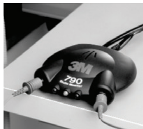
Figure 6: 3M™ Static Monitor 790 attached to equipment chassis
