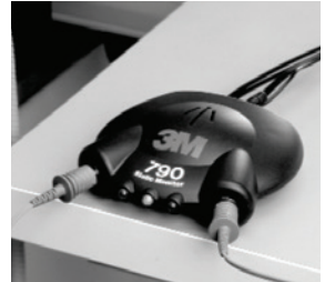
Figure 6: 3M™ Static Monitor 790 attached to equipment chassis
