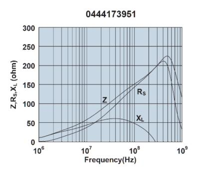
Impedance, reactance, and resistance vs. frequency.
