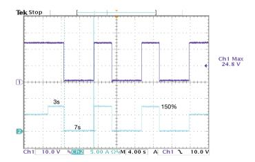
If the peak load is less than 150%, the duration of the peak can be longer than 3s before the output turns off, for example, a peak load of 130% could typically be taken for up to 13s and a peak load of 140% could typically be taken for up to 5s. The off duration is always approximately 7s.
