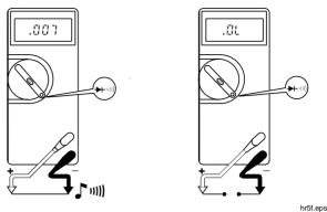
If continuity exists (resistance < 210  $\Omega$ ), the beeper sounds continuously. The meter beeps twice if it is in the Touch Hold® mode.
