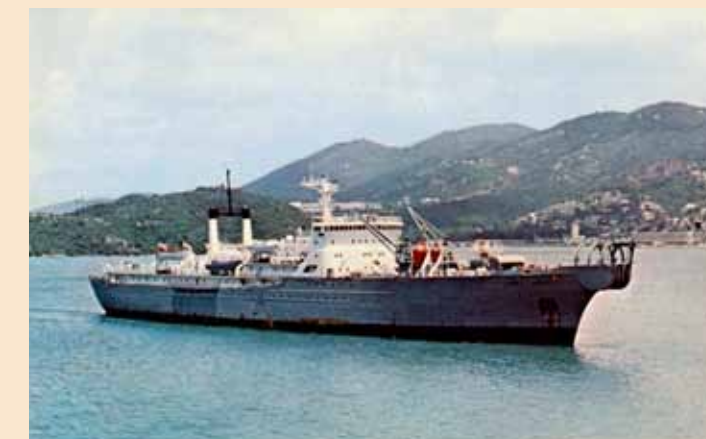
CS Long Lines, a ship designed to lay the Trans-Atlantic fiber optic cable for AT&T. This ship was used to conduct the first deep-sea trials of fiber optic cable in 1982. AT&T laid and opened the first fiber-optic cable across the Atlantic in 1988.
