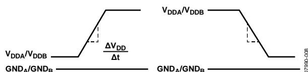
Figure 13. Transient Immunity Waveforms, Output Supplies
