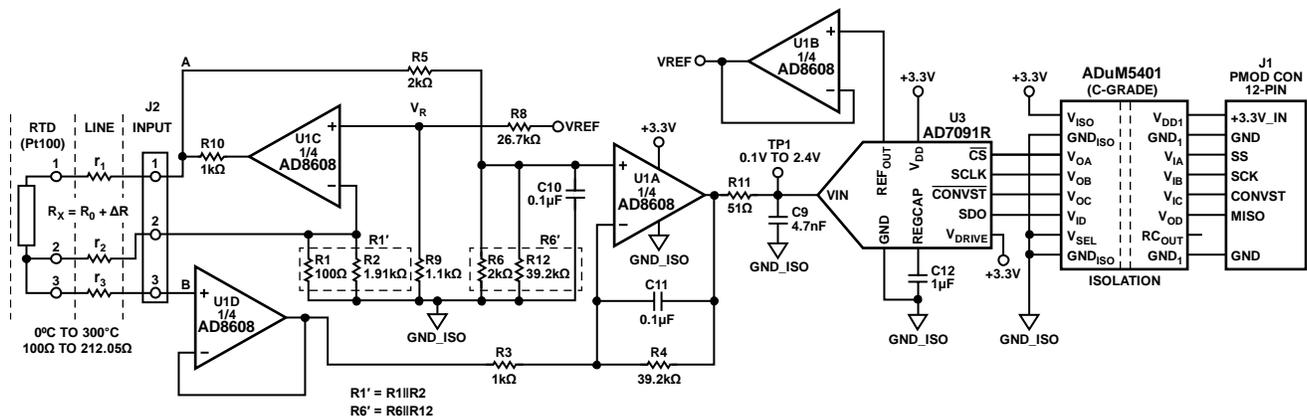
Figure 1. Resistance Deviation to Digital Conversion with Isolation Using Pt100 RTD Sensor
