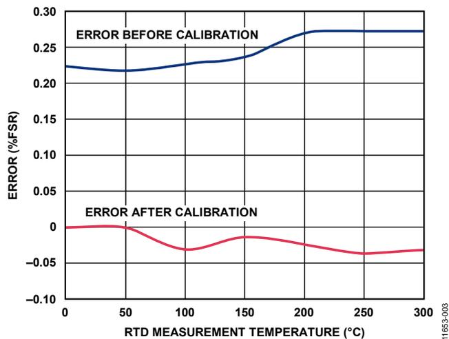
Figure 3. Circuit Error Before and After Calibration
