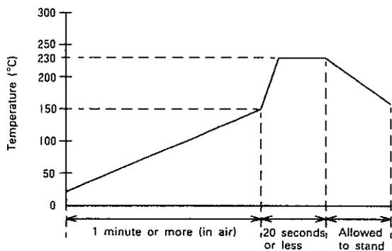
(Note) Complete reflow soldering within 5 seconds at the board surface peak temperature of 240°C or less. The packaging temperature profile varies depending on the board size, type of solder used, and solder thickness.
