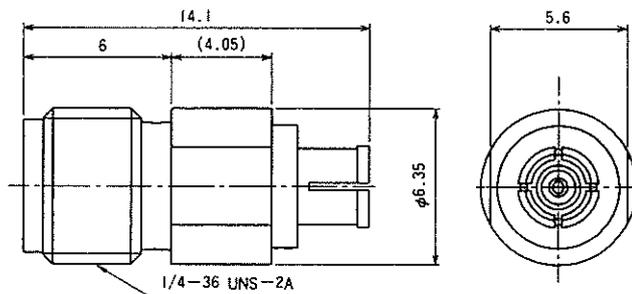
Note: The mated part on the H.FL side cannot be used for any purpose other than performance measurement because there is no lock mechanism.
