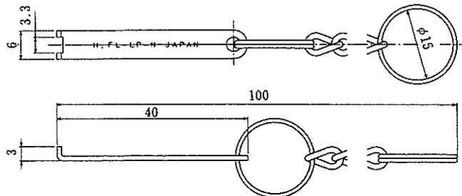
Note: This jig can be used in narrow spaces because it can be inserted from the cable side.
