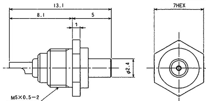
Note: This receptacle is used to inspect the conductivity and withstand voltage of harnesses.
