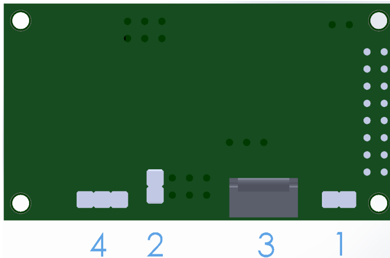
Figure 2: OLED0821 Standard Module Header Locations
