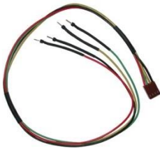
Figure 4: Breadboard Cable (BBC)
