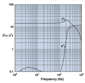
Measured on an 18/10/6mm toroid using the HP 4284A and the HP 4291A.
