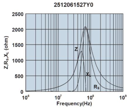
Impedance, reactance, and resistance vs. frequency.
