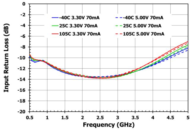
**Figure 29. RFOUT Return Loss versus Temperature (5V Variation)**
