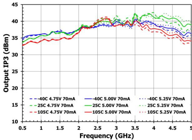
**Figure 8. Output IP3 versus Temperature (5V Variation, 80mA)**
