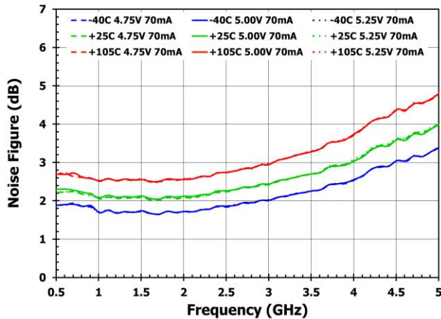
**Figure 36. Noise Figure versus Temperature (3.3V Variation)**
