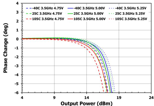
**Figure 23. Gain Compression versus Temperature (5V, 4.1GHz, 70mA)**
