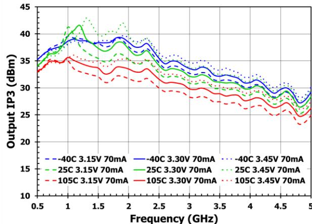
**Figure 10. Output IP3 versus Temperature (3.3V Variation, 40mA)**
