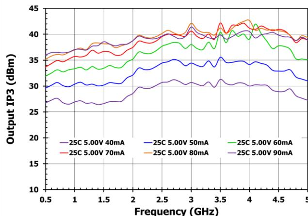
**Figure 12. Output IP3 versus Bias Current (3.3V)**
