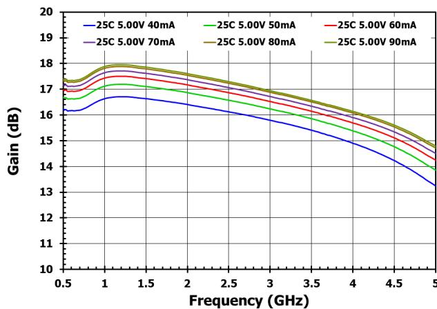
**Figure 6. Gain versus Bias Current (3.3V)**
