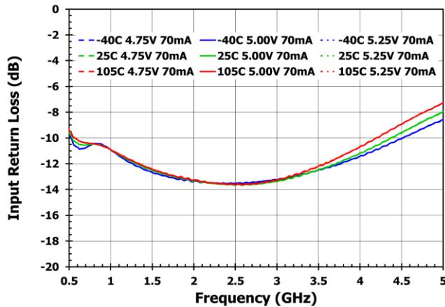
**Figure 28. RFIN Return Loss versus Temperature (3.3V Variation)**
