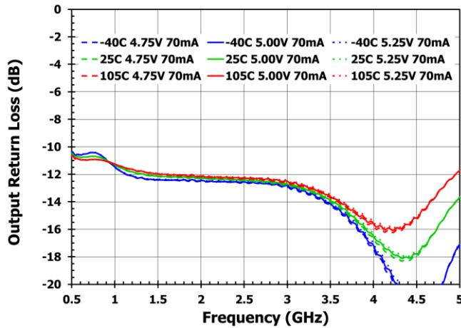
**Figure 30. RFOUT Return Loss versus Temperature (3.3V Variation)**
