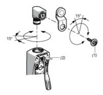
(1) Tightening torque (Min: 1) (Max: 1.5)
