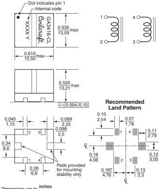
Dimensions are in  $\frac{\text{inches}}{\text{mm}}$
