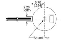
Piezoelectric Buzzer External Drive)
