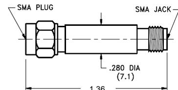
Note: dimensions shown above are for the Male/Female version. The length for the Female/Female version is 1.33 and for the Male/Male version is 1.39.
