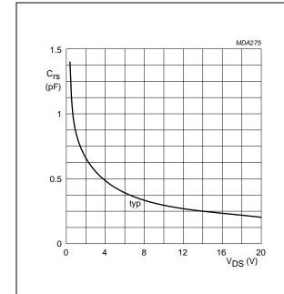
Fig.2  $V_{GS}$  = 0 for BF510 and BF511;  $I_D$  = 5 mA for BF512 and BF513; f = 1 MHz;  $T_{amb}$  = 25 °C.
