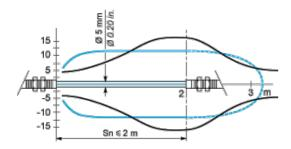
Excess Gain Curves (Ambient temperature: ± 25 °C)
