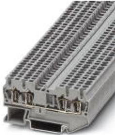
Feed-through terminal block, Connection method: Spring-cage connection, Cross section: 0.08 mm<sup>2</sup> - 1.5 mm<sup>2</sup>, AWG: 28 - 16, Width: 4.2 mm, Color: green, Mounting type: NS 35/7,5, NS 35/15
