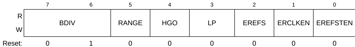
Figure 11-4. ICS Control Register 2 (ICSC2)
