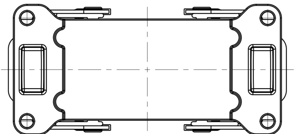
TYPE 3: HIGH CONSTRUCTION + METAL DOUBLE LOCKING,
