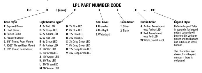
\* 2V LED's are intended for use with an external resistor. See LED voltage chart in appendix for details on the approximate value of the resistor. All green and blue LEDs are recommended for use with translucent button color white only. For super bright LEDs, contact factory.
