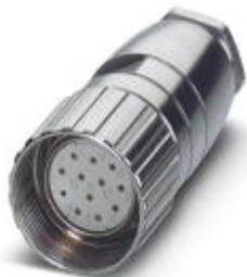
Cable connector, with Pg11 connection thread, straight, shielded: no, Screw locking, M23, No. of pos.: 7, type of contact: Socket, Solder connection, cable diameter range: 8 mm ... 12 mm
