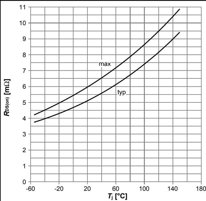
$R_{DS(on)}=f(T_j)$ ;  $I_D=41$  A;  $V_{GS}=10$  V
