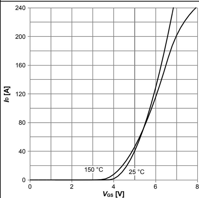
$I_D=f(V_{GS})$ ;  $|V_{DS}|>2|I_D|R_{DS(on)max}$ ; parameter:  $T_j$
