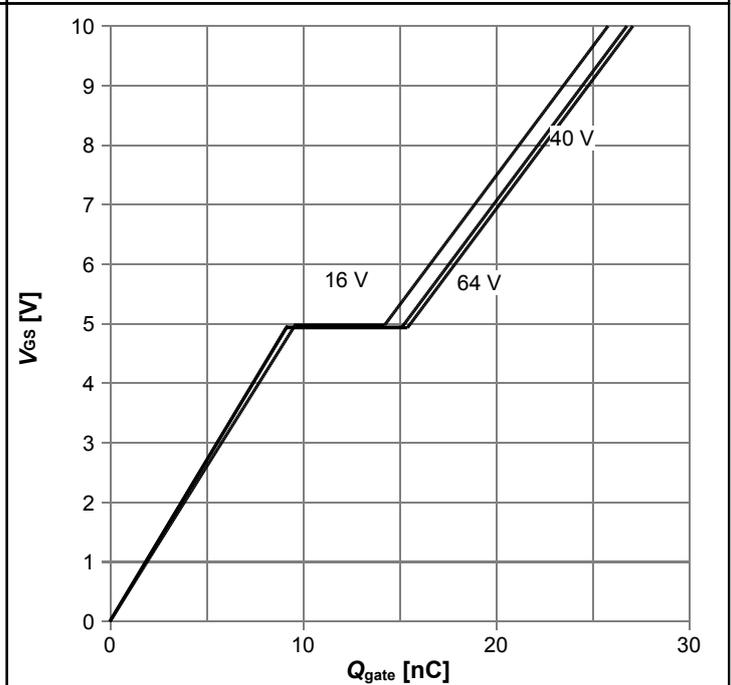
$V_{GS}=f(Q_{gate})$ ;  $I_D=41$  A pulsed; parameter:  $V_{DD}$
