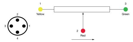
Direction of wiper displacement with shaft extended
