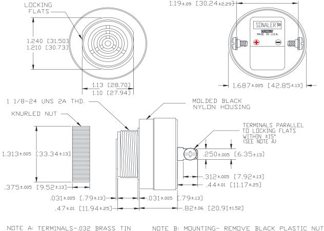
1.25" HOLE PUNCHED IN PANEL, IF ORIENTATION IS NEEDED, NOTE LOCKING SCREW. TWO #6-32 NICKEL PLATED BRASS SCREWS INCLUDED. WILL ACCEPT 1/4"
