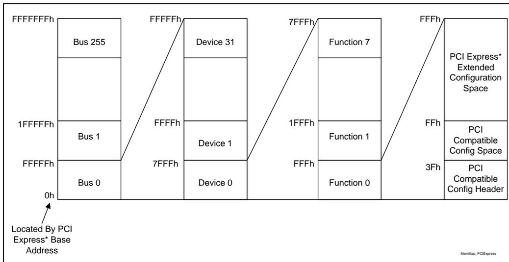
As with PCI devices, each device is selected based on decoded address information that is provided as a part of the address portion of Configuration Request packets. A PCI Express device will decode all address information fields (bus, device, function and extended address numbers) to provide access to the correct register.
