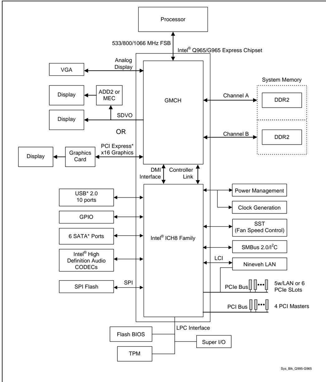
Figure 1-2. Intel® Q963 Express Chipset System Block Diagram Example
